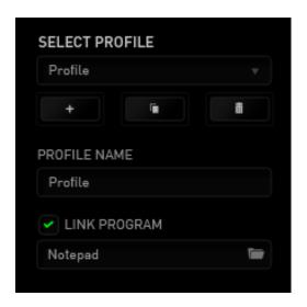
**Profile** contains the default settings of your device. Any changes made within each tab will automatically be saved into the current profile. If you want to rename this profile, you may do so by typing on the field below PROFILE NAME.
