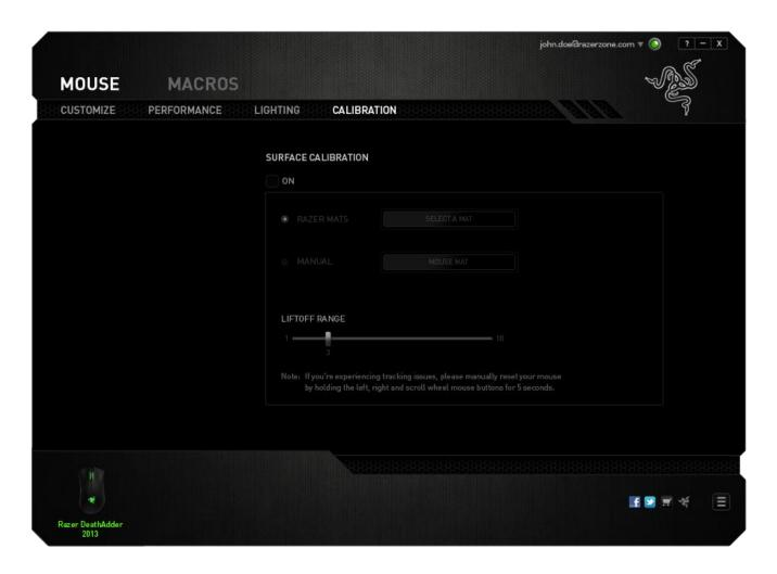
The LIFTOFF RANGE allows you to set the distance in which the sensor stops tracking as it is being lifted away from its mousing surface. To use this feature, you must first activate SURFACE CALIBRATION then choose an appropriate mousing surface.
