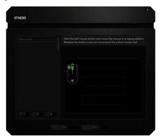
When you have moved through your entire mousing surface, release the left mouse button. This will bring you back to the manual calibration submenu which contains new information regarding your mousing surface.
